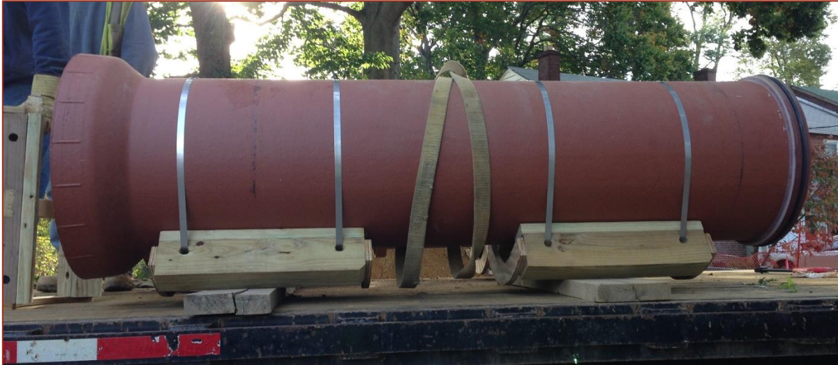
Fig 3: Wood skids attached to 12-inch Bell and Spigot VCP using steel banding.
