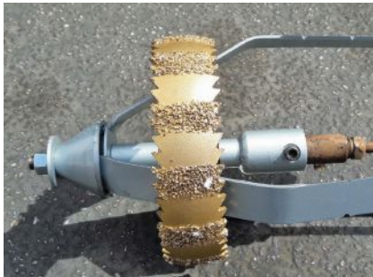
Cutting nozzles are effective for combatting thick roots.
