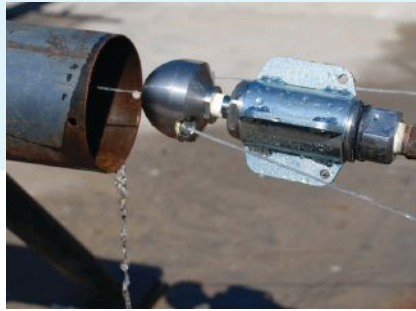
Above left and right are examples of rotary nozzles, which are designed to deliver water throughout the internal circumference of the pipe.
