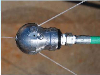
Above left and right are examples of rotary nozzles, which are designed to deliver water throughout the internal circumference of the pipe.
