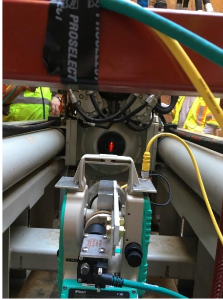
Figure 7: Pilot tube theodolite with integrated camera and visible LED illuminated target.
