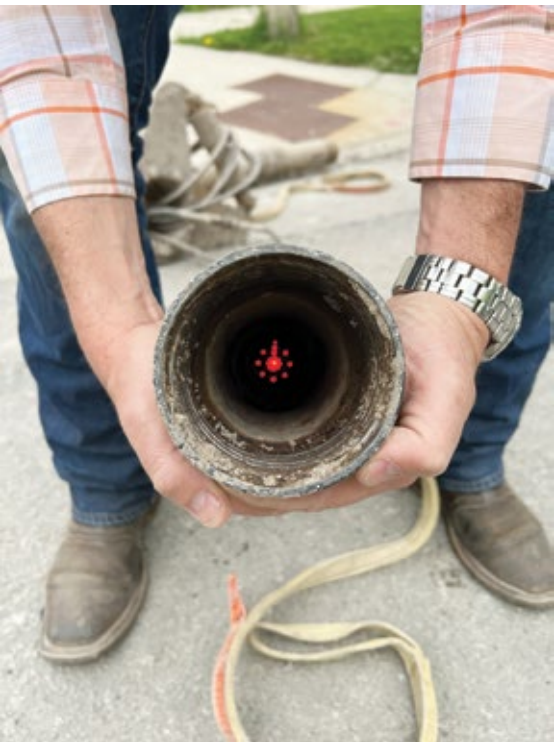
The LED illuminated target is part of the steering mechanism for the pilot tubes
