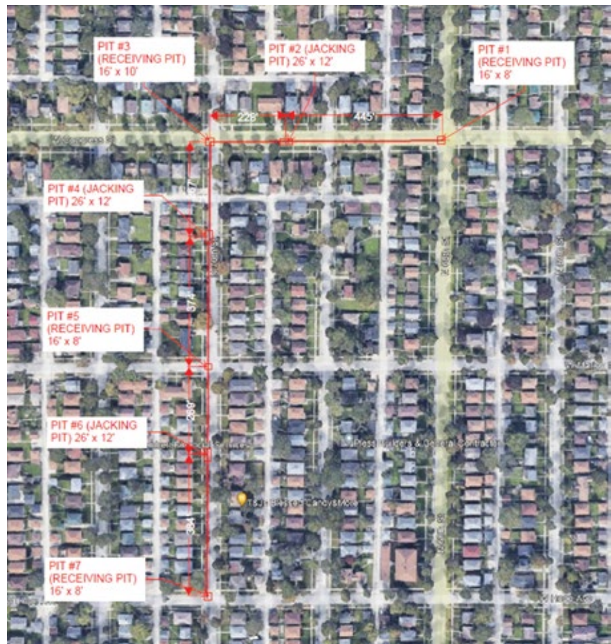
High-density housing was just one of the reasons for trenchless installation on this project
