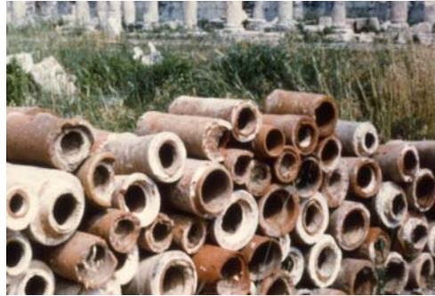
After 2,500 years of service as wastewater pipe, this pipe was returned to service as stormwater pipe and is still in service today.
