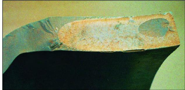
Figure 2 — Void manufactured in wall of PVC pipe (smaller circular area at upper right) which eventually caused fracture to catastrophically propagate.
