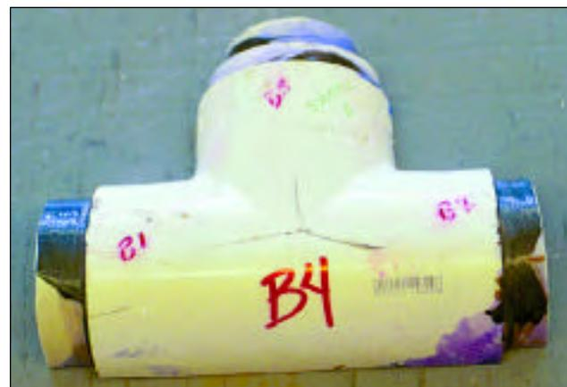
Figure 3 — Cyclic fatigue fracture of PVC tee used in water spraying system.
