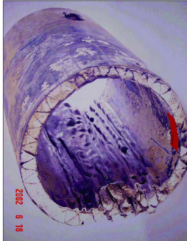
*Figure 1 — Section of ABS truss pipe affected by long-term exposure to drycleaning solvents.*
