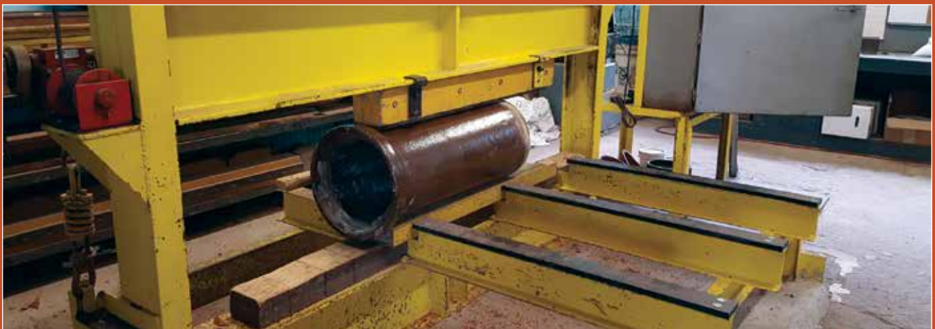
The 120-year-old pipe being tested in the lab at The Logan Clay Products Company. The 3-foot pipe withstood over 5100 lbs. of pressure in the three-edge bearing test.
